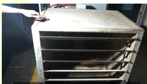
Fig: drying chamber
